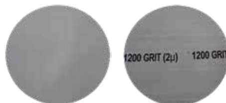
1200 grit (2 micron) front / back side SiC foil
