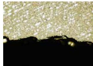
Silicon edge damaged after sectioning with medium grit diamond wafering blade
