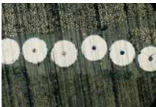
Boron-graphite composite sectioned with fine grit diamond wafering blade. Boron fibers damage minimal.
