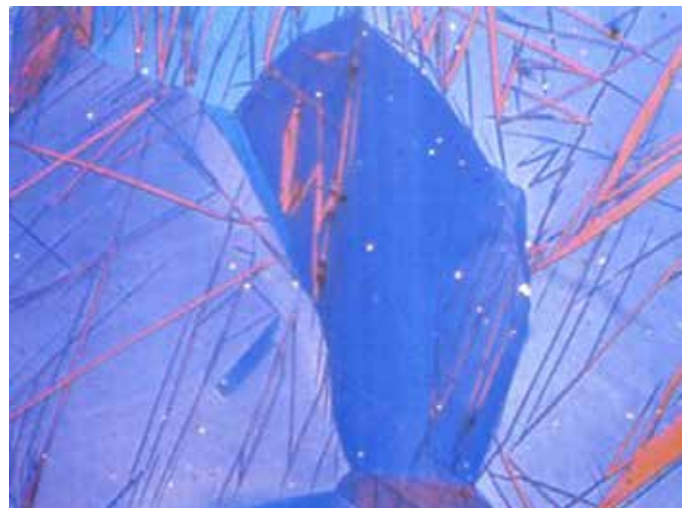
Fe-Ni-Co-Al Alloy, 400X (Polarized Light)
