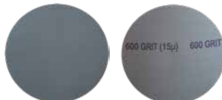
600 grit (15 micron) front / back side SiC foil
