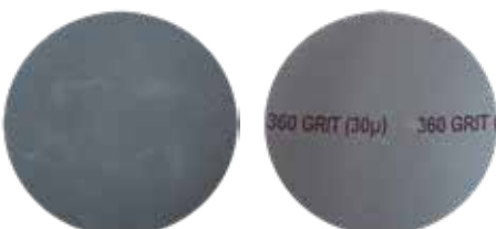
360 grit (30 micron) front / back side SiC foil
