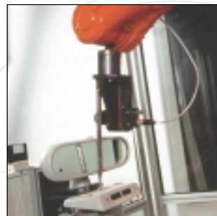
Inspection of rear-view mirror
