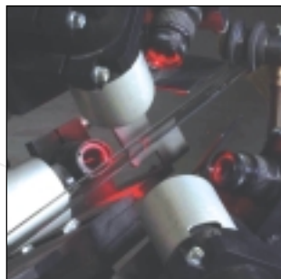
Glass tube inspection
