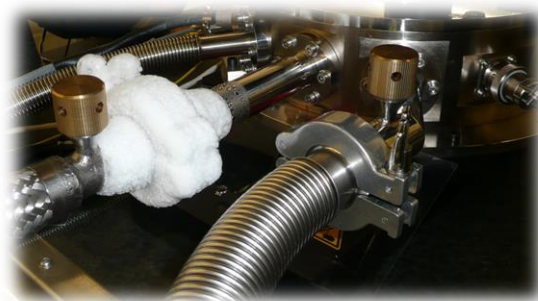
Cryogenic feeding with liquid N2
