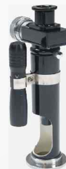
20X Measuring Microscope (With LED light) (#832-213)
