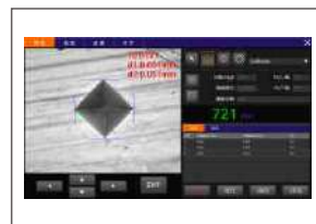
Vickers Measuring System (#821-834)
