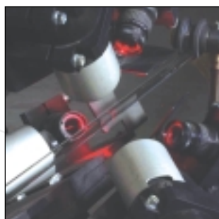
Glass tube inspection
