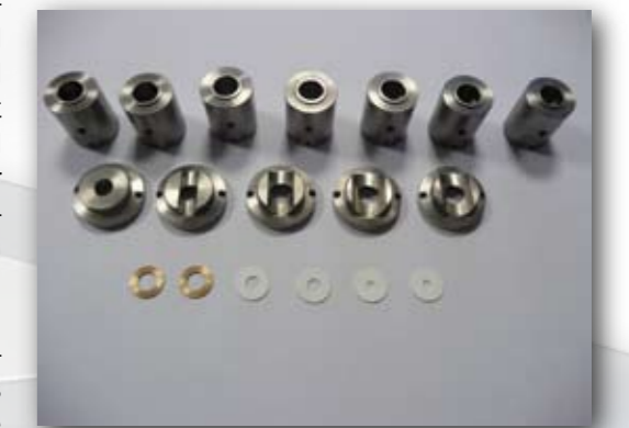
Adaptors and reducer rings allows to analyze even small samples and thin wires
